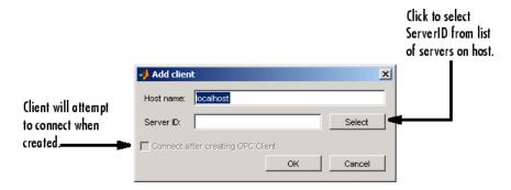
When you supply a hostname, you will be able to select the Server ID from a list, by clicking **Select**. Using the Add client dialog, you can also automatically attempt to connect to the server when the client is created, by checking **Connect after creating OPC Client** before clicking **OK**.
