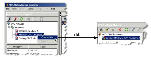
The name of the client (displayed in the **OPC Toolbox Objects** pane) is *Host/ServerID*, where *Host* is the hostname and *ServerID* is the Server ID associated with that client. In this example, the client's name is 'localhost/Matrikon.OPC.Simulation.1'
