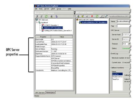
The OPC server properties include diagnostic information, such as the supported OPC Data Access interfaces, the time the server was started, and the current server status.
