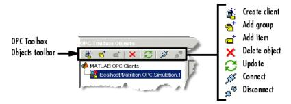
Click **Connect** in the **OPC Toolbox Objects** toolbar. If the client is able to connect to the server, the icon for that client in the **OPC Toolbox Objects** tree will change to show that the client is connected. If the client could not connect to the server, an error dialog will show any error message returned. See "Troubleshooting" on page 1-17 for information on why a client may not be able to connect to a server.
