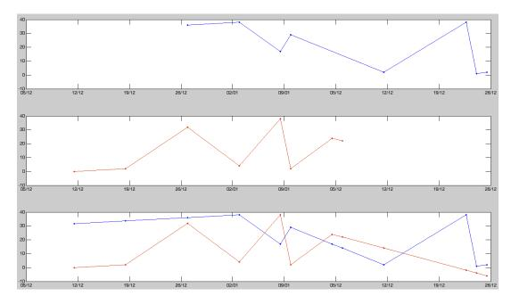
The top two plots above depict two separate data objects. The bottom plot is the result of these two data objects being passed to the tsunion function. You can see that in the bottom plot that each element has been extended to include the timestamps of the other and that values have been extrapolated to satisfy these new timestamps.
