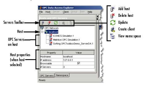
Note that the local host in this example provides three OPC servers. The Server ID for this example is 'Matrikon.OPC.Simulation.1'.
